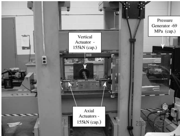
Fig. 2. Hydroforming press at Michigan Technological University capable of 68 MPa of internal pressure and 3600 kN closing force.
