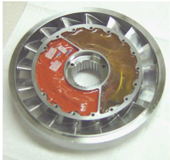
Fig. 11 Stator with cover removed to show telemetry electronics installed in the hub
