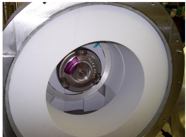
Figure 3. Torque converter dynamometer test cell, from left to right, hydraulic pump, input dynamometer, test fixture and output dynamometer.
