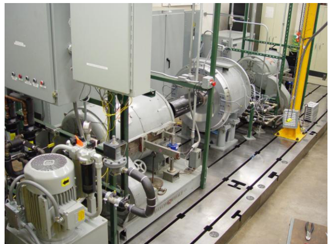
Figure 3. Torque converter dynamometer test cell, from left to right, hydraulic pump, input dynamometer, test fixture and output dynamometer.
