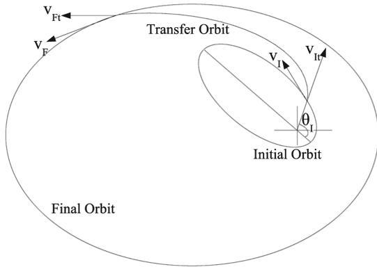
Fig. 1 Geometry for orbit transfer.
