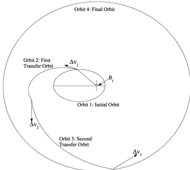
Fig. 2 Three-impulse orbit transfer geometry.
