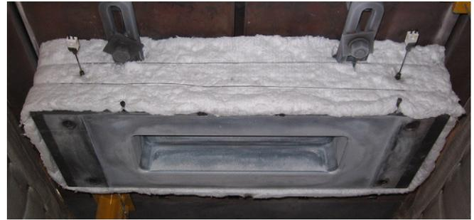
Fig. 1. SPF die with long rectangle forming cavity.
